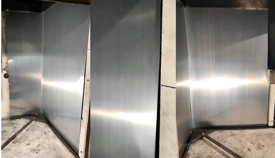
Figure A.1: EN 13823 pre-test photographs
